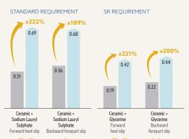
Shoes For Crews outsole Industry standard Slip resistance test according to EN ISO 20344:2021,
